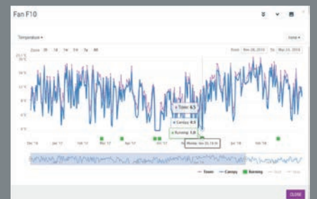
Example report showing tower probe temperature, canopy temperature and running for an individual machine.
