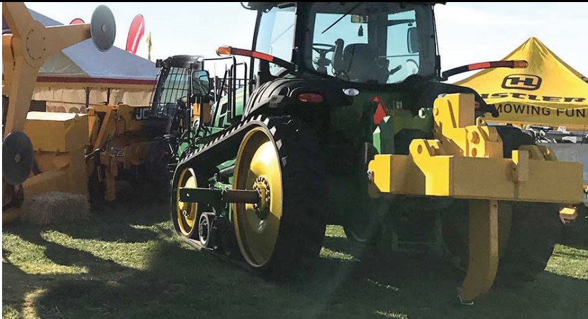
Single ripper - optional to have delving plate with depth to 1 meter
