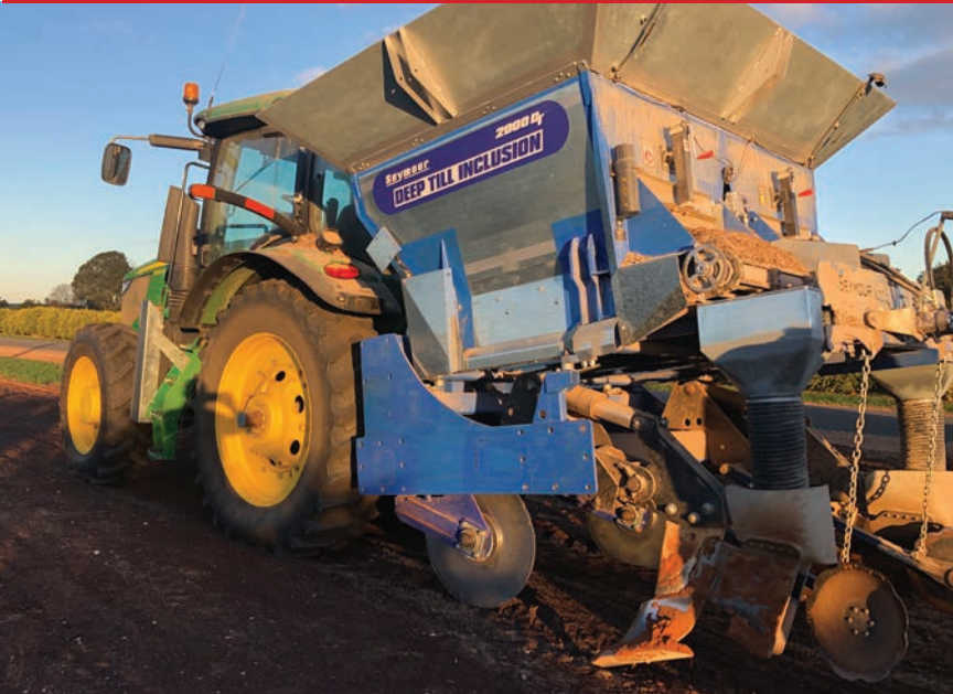
Deep Till Inclusion of manures etc. Large coulters to cut roots. Ripping down to 650mm deep.
