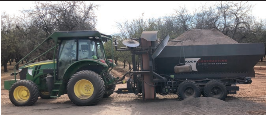
Spreader placing compost and maure into the soil near the drip line mainly in almond orchards. Also a general spreader used in vineyards or citrus orchards. Two machines available with variable rate, and onboard weight scales.
