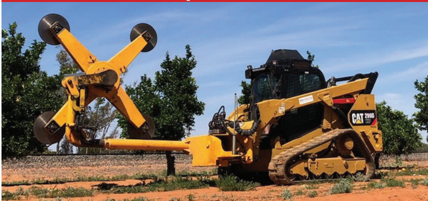
Caterpillar 110hp tracked skid steer attached with a hedger. Capable of hedging tops, slides and skirting. Machine also couples up to a FAE Mulcher.
